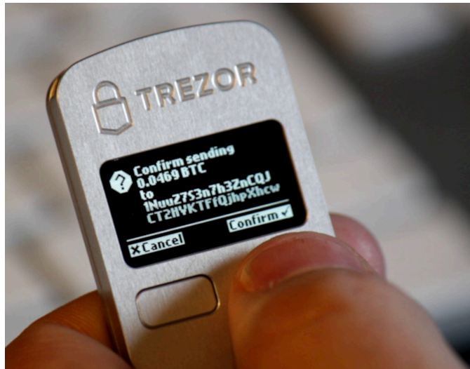
Figure 8.6: A Trezor hardware wallet requesting human confirmation for a transfer.
