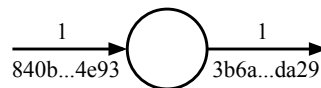
Figure 3.3: A transaction pays from one public key to another. It does not contain real names or other identifying information.
